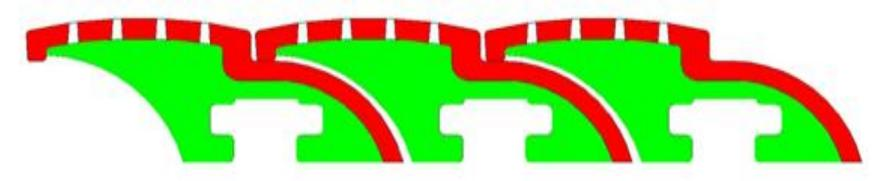
Continuous ash discharge from grate ensures removal of clinkers, if formed, without stopping the boiler.
